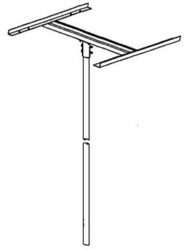
ISOMETRIC VIEW OF PV MOUNTING PIPE
